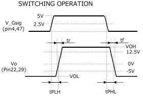
\*RG=1.5Ω, C\_load:0.33uF, f=10kHz, ON Duty=50%
