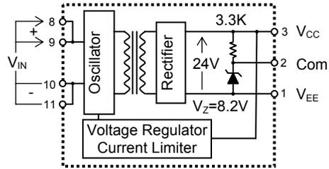
**Circuit Explanation:** The BG2C is a basic two channel gate driver designed around the recommended application circuits for the Powerex VLA507 and VLA513 hybrid IGBT gate drivers in combination with either VLA106-15242 or VLA106-24242 isolated DC to DC converters.
